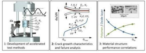
Fracture mechanics-based approach
