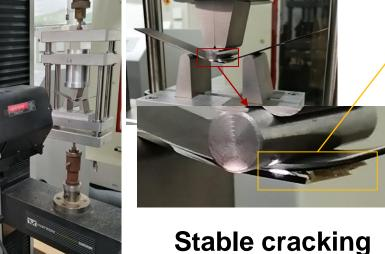
→ Need to add a better failure description to the model: propagation With the microscope
