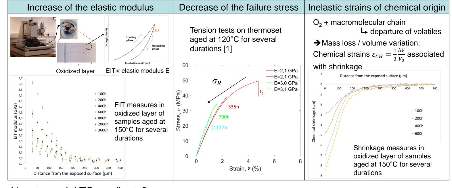
How to model TO gradients? Use of a phenomenological parameter representative of TO progress  $\gamma$  [2]
