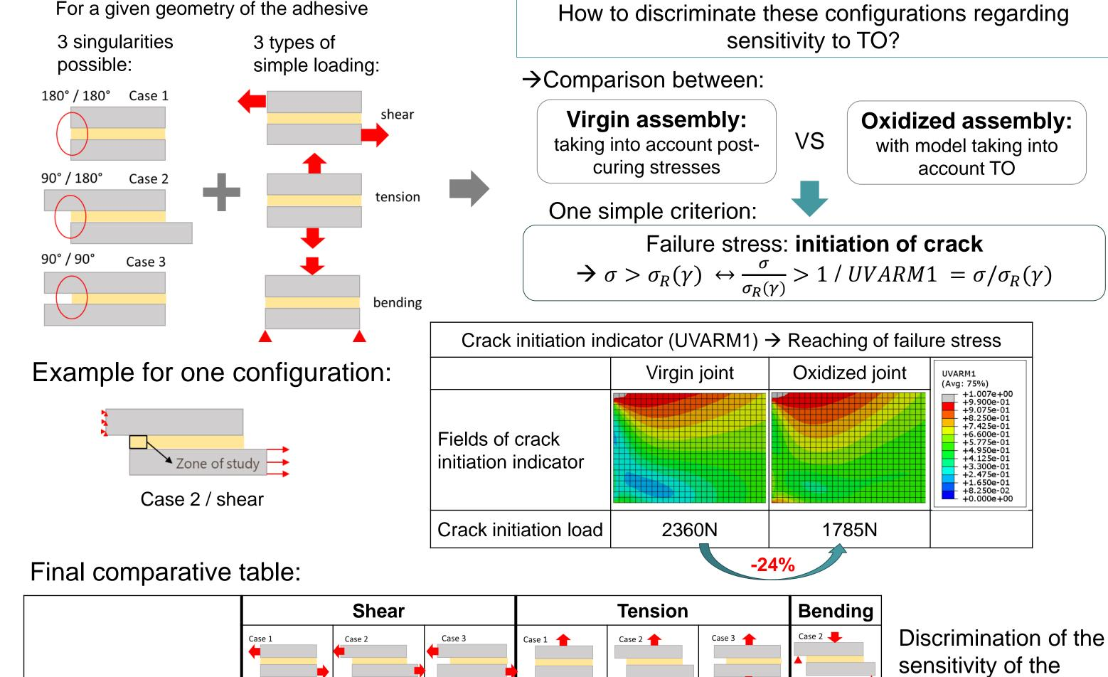
Numerical analysis on crack initiation through a simple criterion: not enough to conclude → Need to consider other experimental aspects
