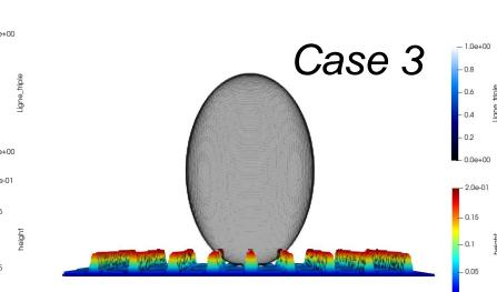
To represent the effects of the deposit method different initial states are studied (shape, position along z axis)
