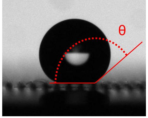
Contact angle along transversal plan
