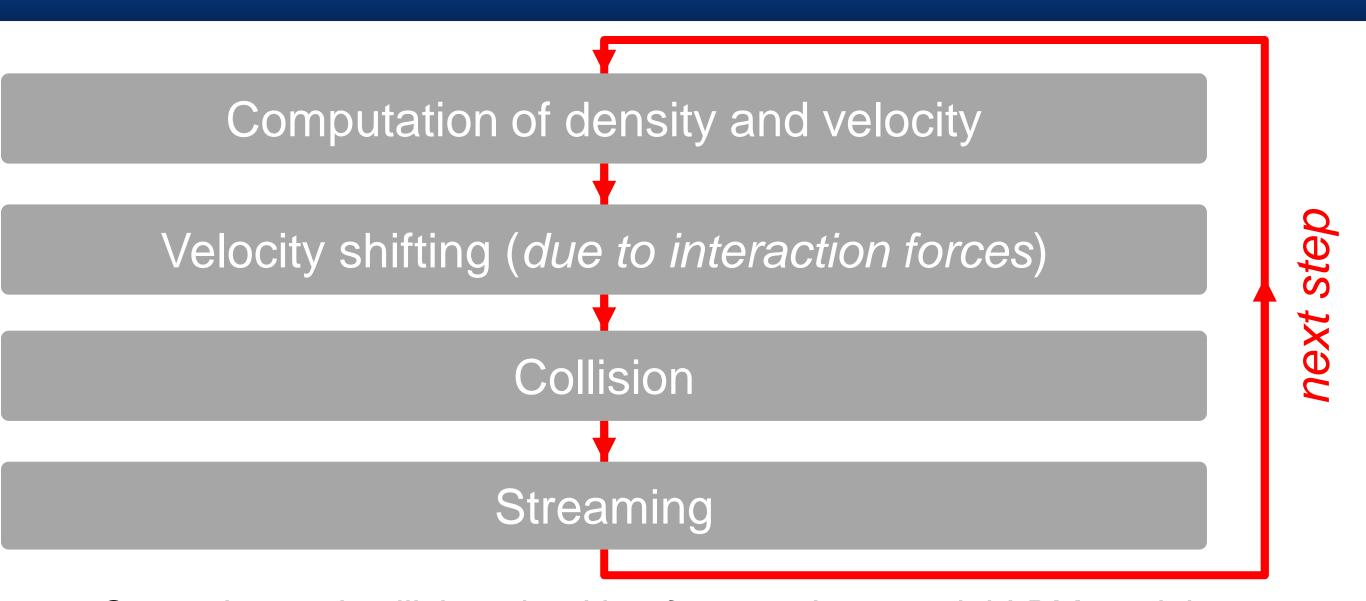
Streaming and collision algorithm for pseudo-potential LBM model
