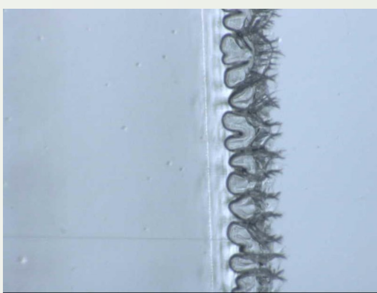
Peeling front from bottom on homogeneous substrate
