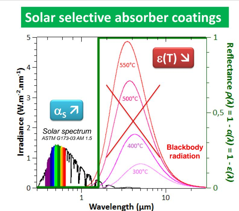
For an ideal solar receiver, spectral reflectance  $\rho(\lambda)$
