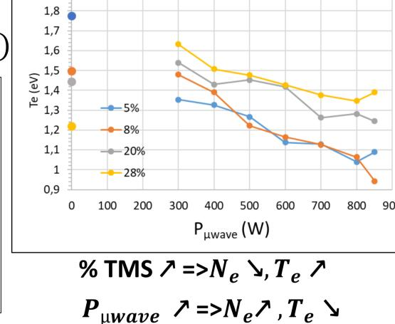
Effect of ECR MW sources: Significant modification in plasma parameters
